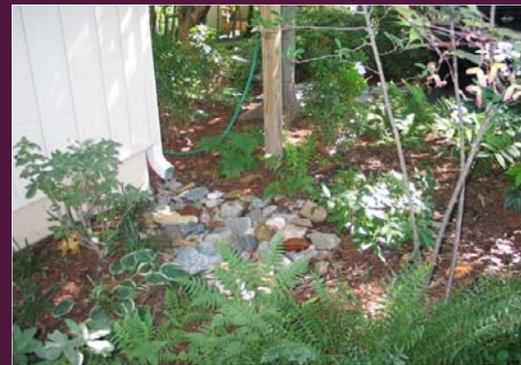
A disconnected downspout can be directed to a gravel or vegetated area to capture the water. It is important to direct the downspout away from the house to ensure that water does not pool next to your foundation.
