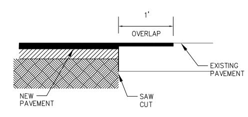
NOTE: NEW PAVEMENT THICKNESS TO MATCH EXISTING PAVEMENT SECTION.
