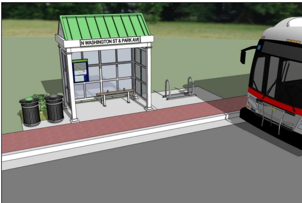
Figure 4: Typical Bus Shelter Described in the City's Bus Stop and Bus Shelter Master Plan (Source: City of Falls Church Comprehensive Plan, Chapter 7: Transportation: "Mobility for All Modes")
